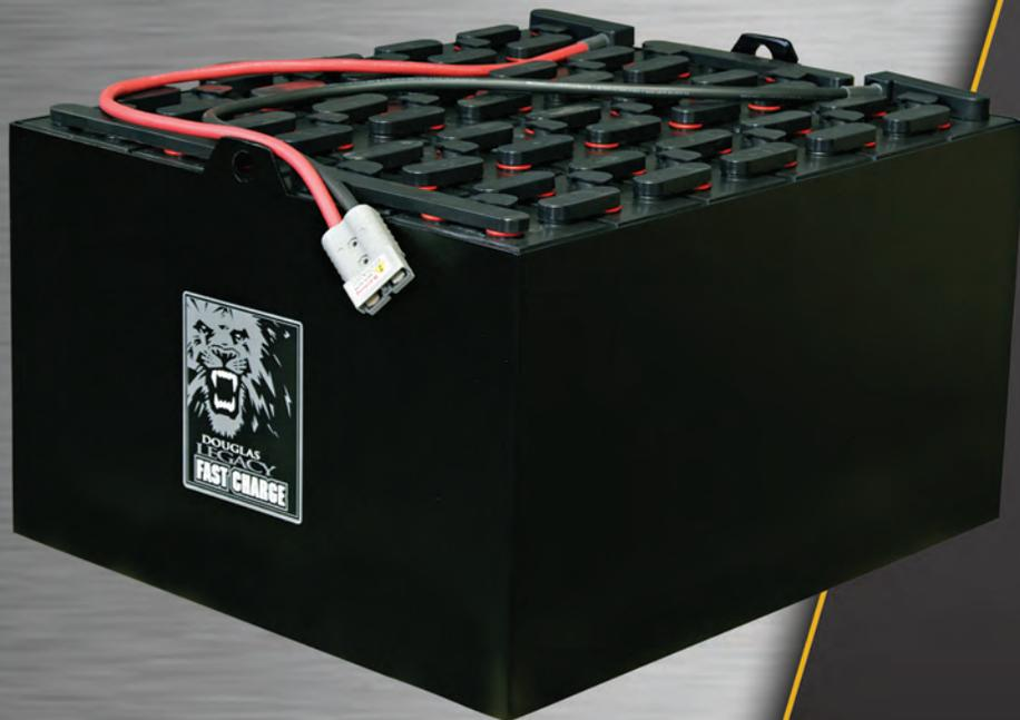
The proven Douglas<sup>™</sup> High Performance Battery design is enhanced for higher charge rates and increased daily ampere hour throughput demanded by opportunity charging applications. The Douglas Legacy<sup>®</sup> Fast Charge battery is designed to accept charge rates up to 25% of the battery's rated capacity.
