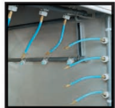
Multi-directional air and water nozzles; Non-metallic air and water lines
