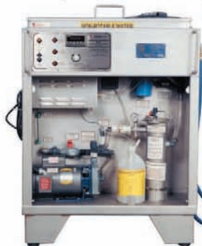
LNC/Ozone auto injection system
