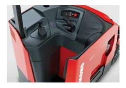
The ergonomically designed compartment and single, low-force deadman pedal reduce operator fatigue and enhance comfort.
